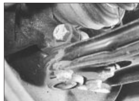
7.3 Track control arm balljoint and clamp bolt
