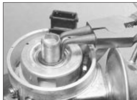
7.4a Remove the locking ring and rotor . . .
