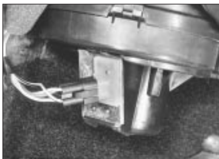
9.3 Blower unit and wiring connection
