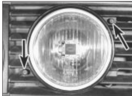
7.4 Foglight beam alignment adjuster screws (arrowed)
