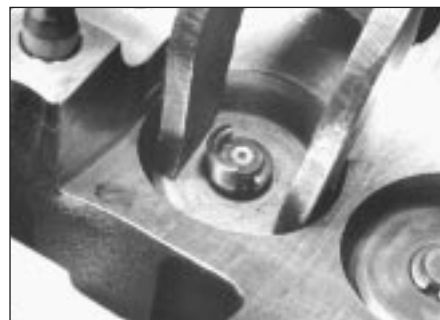
12.12c . . . and valve collets
