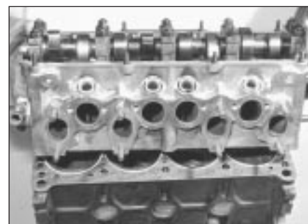
34.3a Lowering cylinder head onto block
