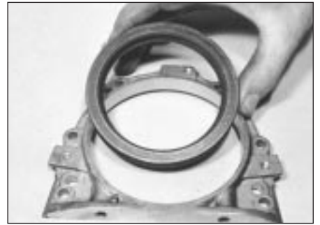
14.14 Remove crankshaft rear oil seal from housing
