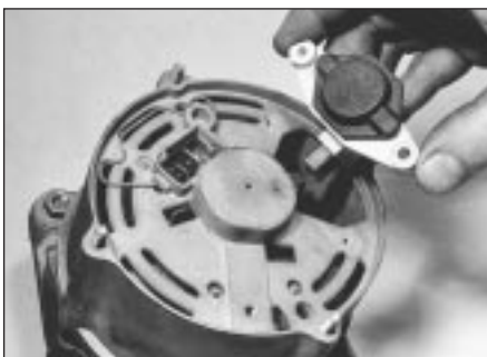
8.3 Removing voltage regulator and brush assembly
