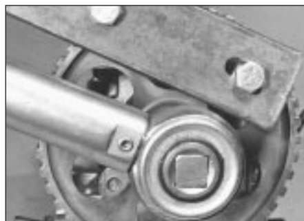
35.5 Method of tightening camshaft sprocket bolt
