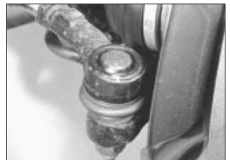
28.2 Inspect balljoint dust covers
