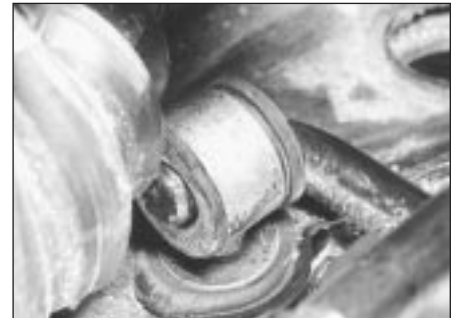
4.5 Anti-roll bar location in eye bolt
