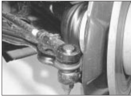
15.1 Right-hand adjustable balljoint
