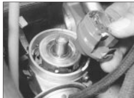
7.3a Pull free the rotor . . .
