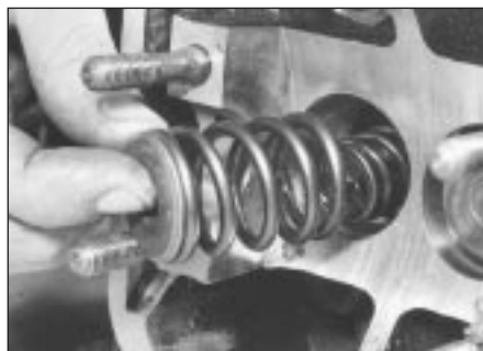
12.12b Locating valve springs and cap . . .
