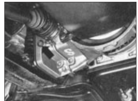
35.10 Final drive unit oil filler/level plug (arrowed)
